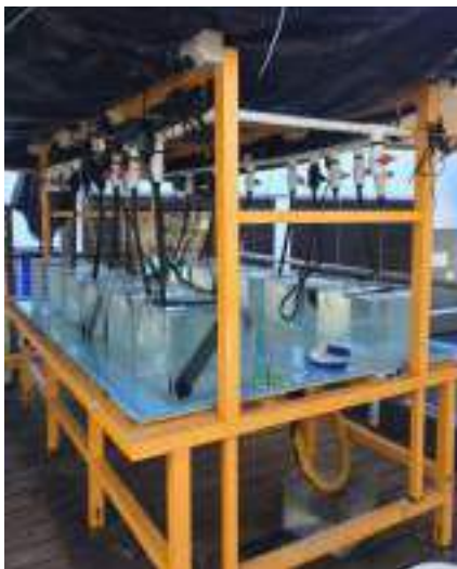
Figure 3. Experimental setup for algae treatment tanks. Twelve 125L flow-through tanks arranged beneath a shade screen to equalize natural light exposure. Tanks were randomly assigned one of four treatments: Control (C), increased light (L), increased temperature (T), and both increased light and temperature (B). There were three replicate tanks for each treatment. Tanks were filled with Laurencia intricata macroalgae and cultured for 5d under treatment conditions. Water for tanks was pumped directly off the reef flat at Heron Island Research Station where the algae was collected. Tanks and equipment were monitored daily to ensure proper functioning.
