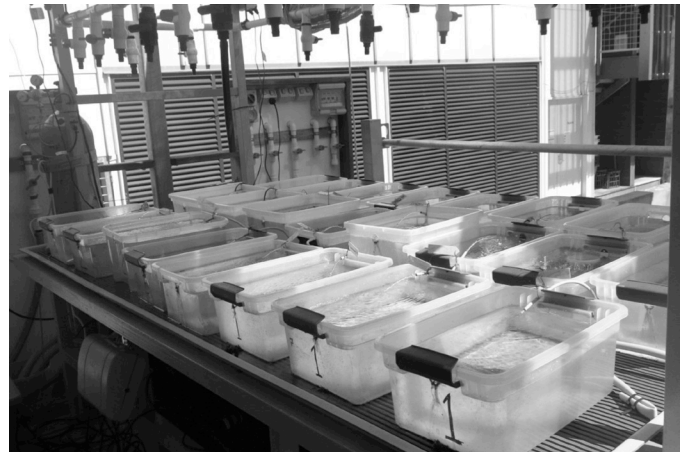
Figure 2. The ocean acidification tank set up on an outdoor deck at Heron Island Research Station. The large pH and heat-controlled sumps are located under the table.
