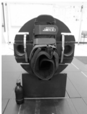
Fig. 2. Image of Knee Rotation Device (KRD). A weight of 1.83 kg applies a 3.51 N torque, rotating the platform axially.
