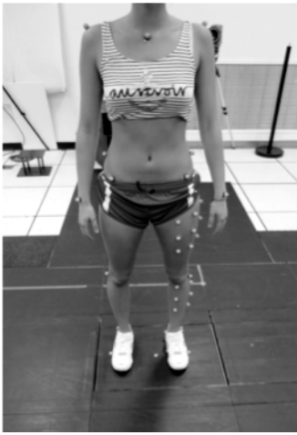
Fig. 1. Subject with reflective PCT markers used for motion tracking with Qualysis.
