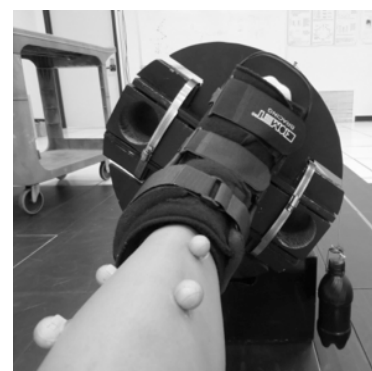
Fig. 4. Image of weight applied to KRD. Motion capture cameras detect changes in position of the reflective markers on the tibia and femur to calculate the knee rotation.
