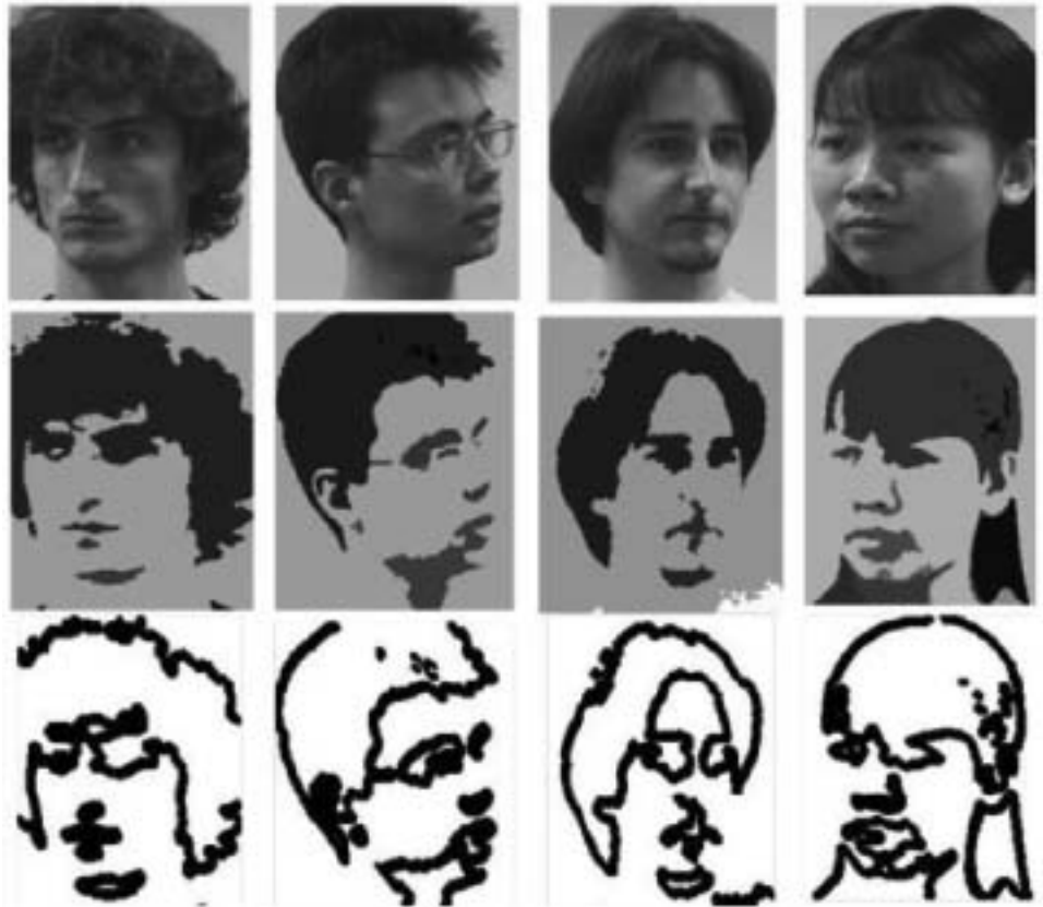
Fig. 6 NPR results for Pointing Database (top to bottom): original image, region segmented image, stroke rendered image.
