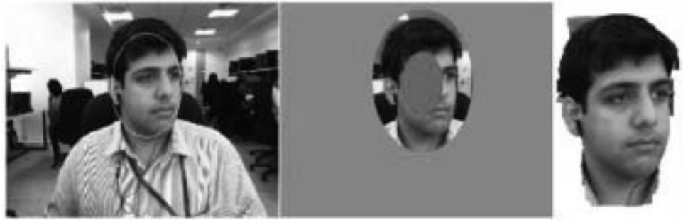
Fig. 10 Elliptical head tracker + GrabCut (left to right): Elliptical head tracker output, Automatically marking sure foreground and background region guided by the ellipse, GrabCut output.
