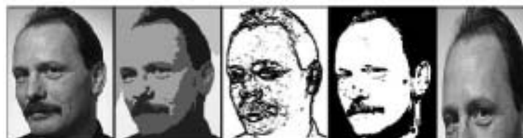
Fig. 2 Various forms of image abstraction (left to right): original image, color segmentation image, contours image, skin detector output, cropped upper face.
