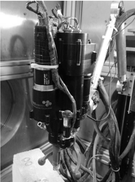
Fig. 1 The Honeybee SASSI, a prototype for MSR, was used for all tests. It is equipped with the full face powder acquisition bit. The SASSI is a rotary-percussive drill, although percussion was disabled during these tests. The arm and the translation stage can be seen in the right of the image.
