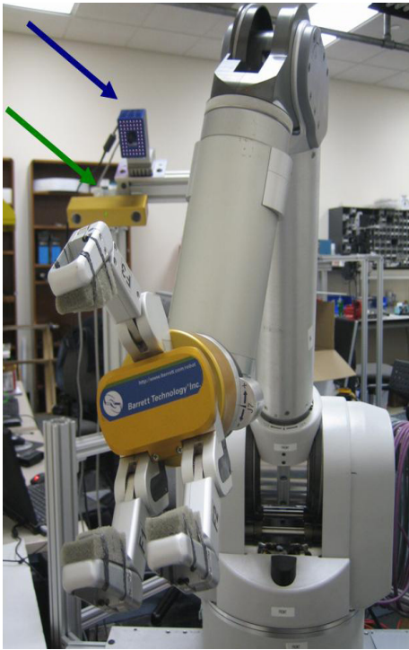
Figure 2: STAIR. 7-dof Barrett WAM Arm and 4-dof 3-fingered BarrettHand with “open” spread pictured. The spread can be “closed” such that all 3 fingers will be at the top. Vision system mounted on robot frame; blue arrow marks SwissRanger, green arrow marks Bumblebee2.
