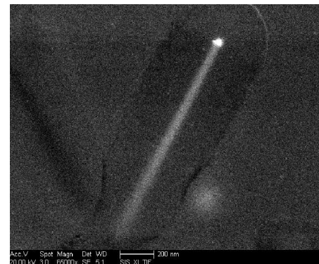
This is an image of a germanium nanowire with the gold catalyst particle still attached to the tip surrounded by silicon oxide. This image was taken under SEM after CMP and cleaning.
