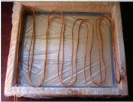
Shower Drain Heat Exchanger – Paul Kreiner
