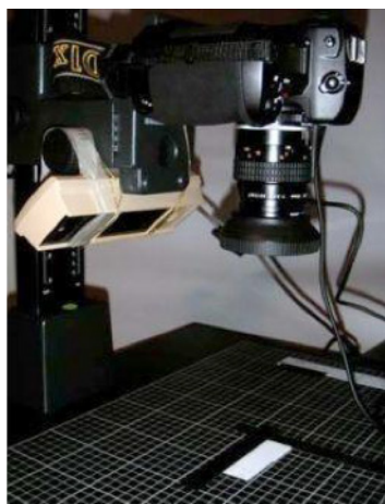
Figure 2. Digital photography of assays. Setup for digital photography of assays. The camera and white light lamp were attached to a stand to ensure a constant distance from the substrate.
