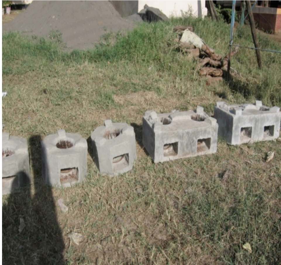
IMAGE 2. ICS without chimneys. Locally made ( Dr. Mwasha Stove ).
