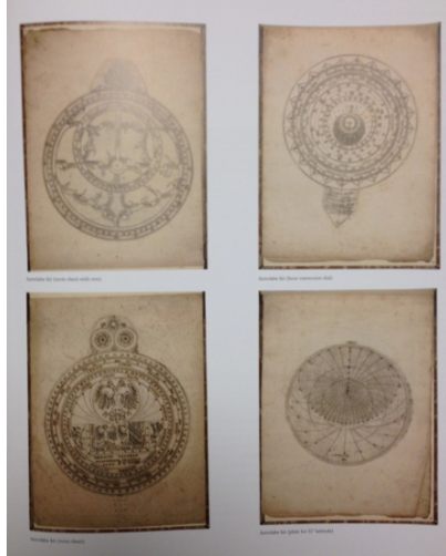
FIGURE 3. Four paper drawings of Hartmann's astrolabe kit. Top left image – recto sheet with rete; top right – hour conversion dial; bottom left – verso sheet; bottom right – plate for 51° latitude. Reproduced from Dackerman, Prints and the Pursuit of Knowledge in Early Modern Europe , 313.
