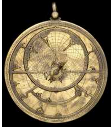
FIGURE 1. This is understood to be the earliest Western astrolabe in the Oxford collection. Muslim influences are seen in the design of this astrolabe's rete, and it may have been made in Spain, ca. 1260.
