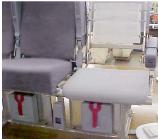
Figure 4. Above is a seat model built with the Dymetrol suspension membrane, which eliminates the need for additional seat pans and saves volume. Reprinted from Acme Mills.
