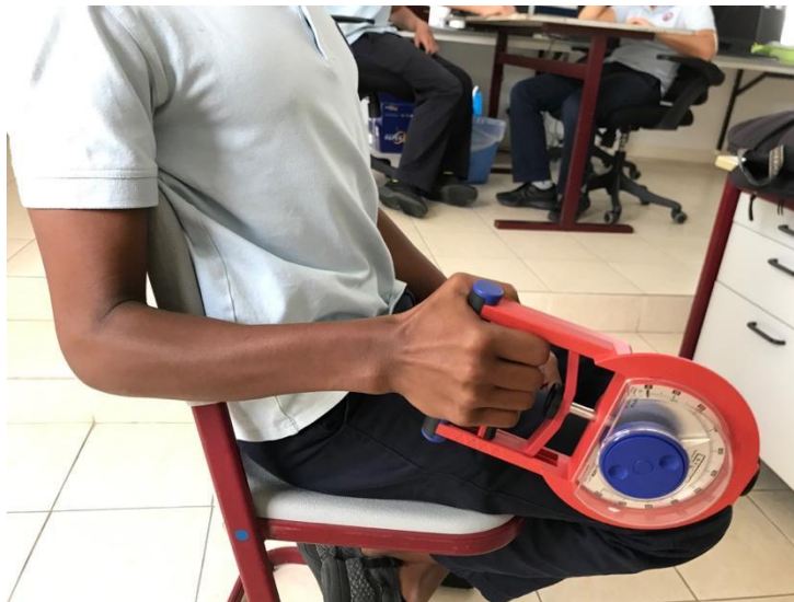
APPENDIX D. Participant using dynamometer at right angle to measure strength, pressing down for 5 seconds at maximum effort.
