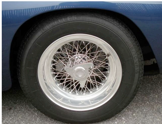
FIGURE 7. A Borrani wire wheel including the spinner on a 1964 Ferrari 250 GT “Lusso.”
